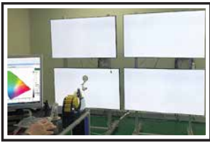
Factory tuning color calibration of white balance
